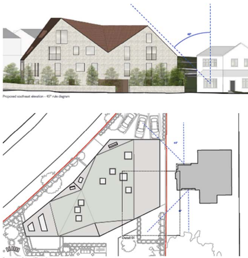
Figure 10- 45 degree test on 218 Brighton Road
